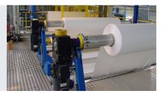
The automatic laminating machine is suitable for felt, textile, paper and film applications. Continuous unwinding units ensure a constant production.
